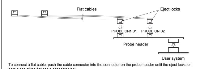
both sides of the flat cable connector lock.
