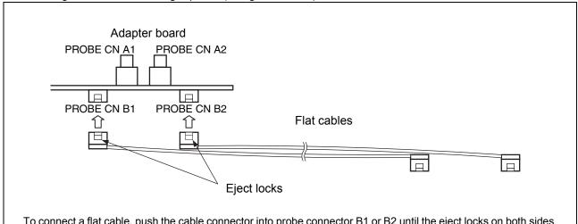
To connect a flat cable, push the cable connector into probe connector B1 or B2 until the eject locks on both sides of the flat cable connector lock.
