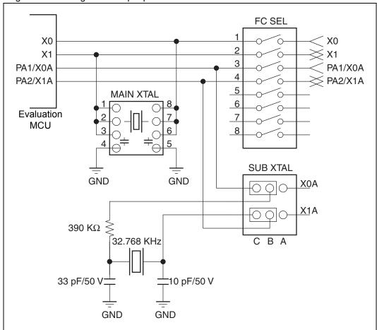
Figure 3-3. Configuration of peripheral circuits for the clock circuit
