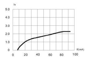
Fig. 2 Relative Luminous Intensity vs. Forward Current
