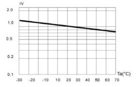
Fig. 5 Relative Luminous Intensity vs. Ambient Temperature
