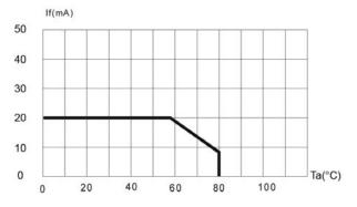
Fig. 6 Maximum Forward Current vs. Ambient Temperature
