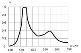
Fig. 4 Relative Luminous Intensity vs. Wavelength
