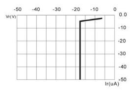
Fig. 3 Reverse Current vs. Reverse Voltage
