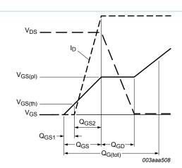
Fig. 15. Gate charge waveform definitions
