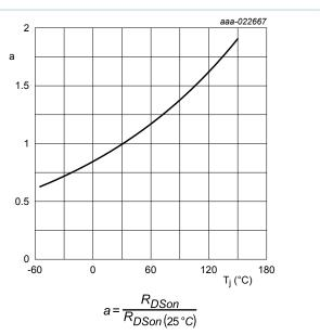
Fig. 11. Normalized drain-source on-state resistance as a function of ambient temperature; typical values
