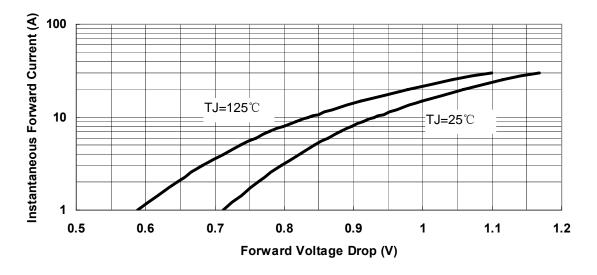
Fig.3-Typical Instantaneous Forward Voltage Characteristics
