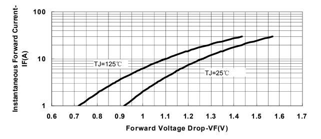
Fig.3-Typical Forward Voltage Drop Characteristics
