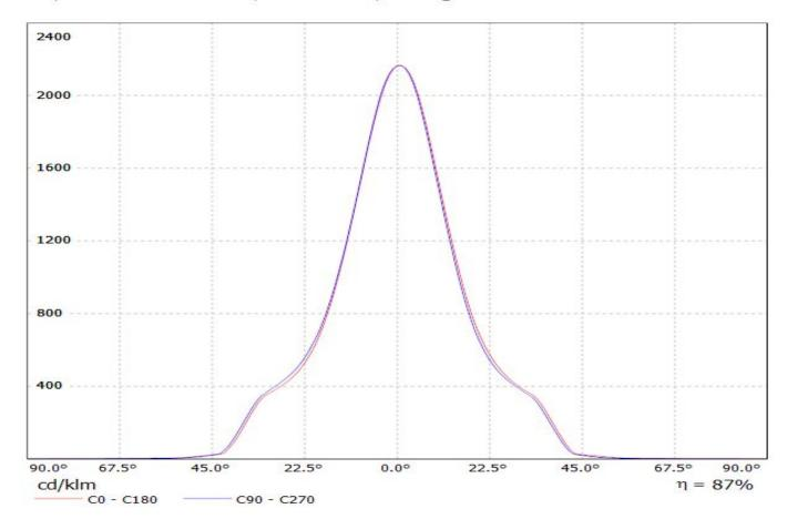
Luminaire: LEDiL Oy CN12645\_LENINA-M\_(Luxeon\_CoB\_1208) Eff: 88 % Lamps: 1 x Luxeon CoB 1208 (LHC1-3080-1208) 1065Im@250mA CCT=3000K P=8.3W I=250mA
