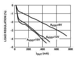
FIGURE 8.  $V_{BOOST}$  LOAD REGULATION AT  $V_{IN} = 5V$  (P MODE)
