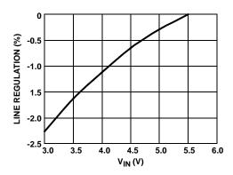
FIGURE 10. VBOOST LINE REGULATION (P MODE)
