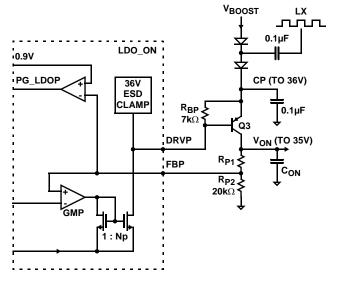
FIGURE 28. VON FUNCTIONAL BLOCK DIAGRAM
