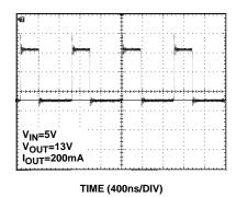
FIGURE 22. LX WAVEFORM - CONTINUOUS MODE
