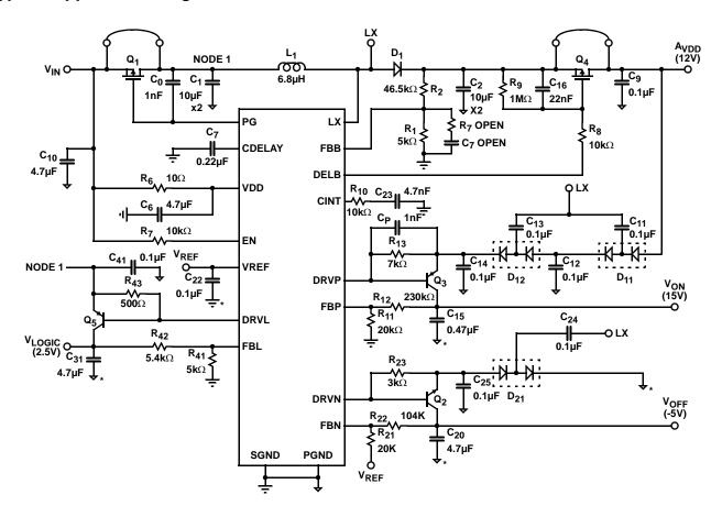
NOTE: The SGND should be connected to the exposed die plate and connectd to the PGND at one point only.
