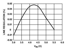
FIGURE 9. VBOOST LINE REGULATION (PI MODE)
