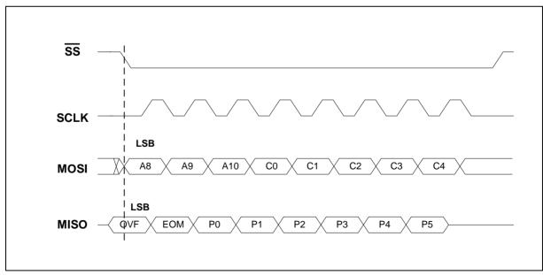
**FIGURE 6: 8-BIT COMMAND FORMAT**
