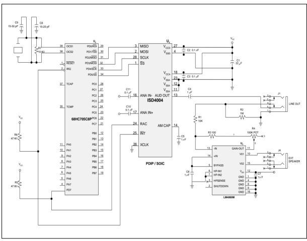
FIGURE 9: APPLICATION EXAMPLE USING SPI
