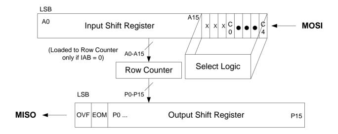
FIGURE 3: SPI INTERFACE SIMPLIFIED BLOCK DIAGRAM
