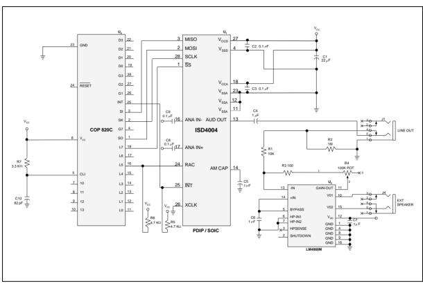
FIGURE 10: APPLICATION EXAMPLE USING MICROWIRE
