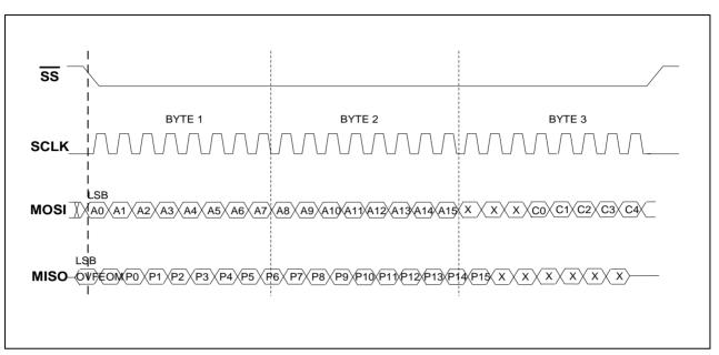
**FIGURE 7: 16-BIT COMMAND FORMAT**
