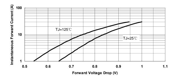
Fig.3-Typical Instantaneous Forward Voltage Characteristics
