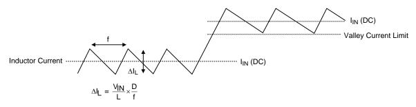
Figure 4. Inductor Currents In Current Limit Operation
