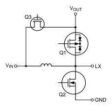
Figure 2. Boost Converter With Bypass Mode
