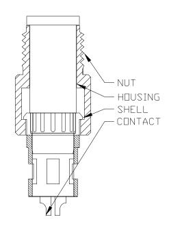
MATERIAL TPU, BLACK HOUSING: CONTACT: BRASS NUT: BRASS SHELL: BRASS FINISH CONTACT: GOLD PLATED □VER 50μ"NICKEL NUT: NICKEL PLATED SHELL: BRIGHT TIN PLATED ELECTRICAL RATED CURRENT: 1Α RATED VOLTAGE: 60V INSULATION RESISTANCE: 1000 M□hms MIN.
