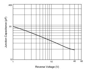
Figure 5. Typical Junction Capacitance
