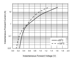
Figure 2. Typical Instantaneous Forward Characteristics
