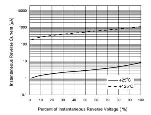
Figure 4. Typical Reverse Characteristics
