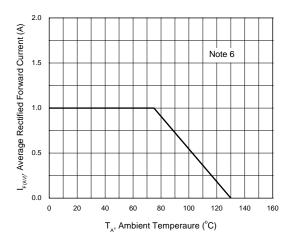
Figure 1. Forward Current Derating Curve
