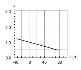
Fig. 6 Relative Luminous Intensity vs. Temperature
