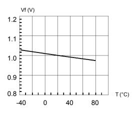
Fig. 5 Forward Voltage vs. Temperature
