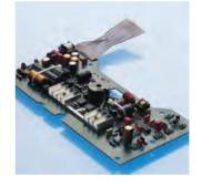
The circuit board above shows punched parts interfacing screwmounted transistors to a finned heat sink.
