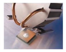
TIC 4000 is a thermally conductive grease compound designed for use as a thermal interface material between a computer processor and a copper-based heat sink. Other high watt density applications will benefit from the extremely low thermal impedance of TIC 4000.
