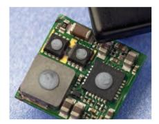
LIQUI-FORM 2000 is a high thermal conductivit y liquid formable material designed for demanding applications requiring a balance between dispensability, low component stresses during assembly and ease of rework.
