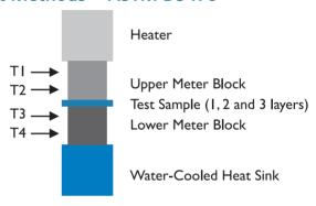
2 in. diameter stack (ref. 3.14 in.2) - 10-500 psi, 1 hour per layer
