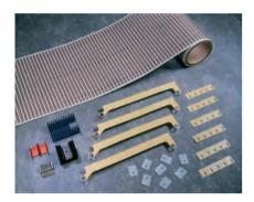
POLY-PAD K-10 is a composite of film coated with a polyester resin. The material offers exceptional thermal performance for your most critical applications with a thermal resistance of 0.2°C-in.²/W as well as excellent dielectric strength.
