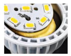
Gap Filler 1500LV is a two-part, high performance, thermally conductive, liquid gap filling material. This material offers the high temperature resistance and low modulus of a silicone material with significantly lower levels of silicone outgassing for use in silicone-sensitive applications.
