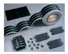
BERGQUIST Q-PAD 3 is a grease-only replacement that does away with contamination of electronic assemblies and reflow solder baths. Q-PAD 3 may be installed prior to soldering and cleaning with confidence. When clamped between two surfaces, the elastomer conforms to surface textures, thereby creating an air-free interface between heatgenerating components and heat sinks.
